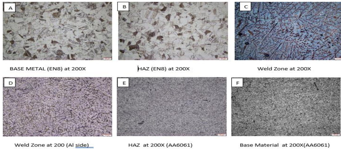
Figure 4.2 : Sample-1 micro structure with different specimens in 60 Amps
