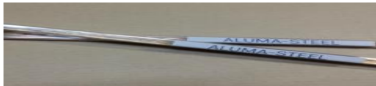
Figure 3.3: showing welding rod- filler rod
